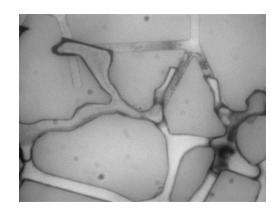
Figure 4: Clogged pores and channels at 300°F
