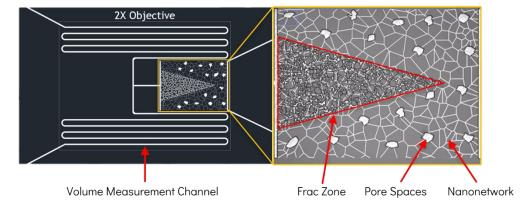
Figure 1. Schematic of the microfluidic analogue used for screening the products. Left is the CAD design of the model. Right is the actual fabricated analogue under the bright-field microscopy. The volume measurement channel is designed to accumulate the produced oil and measure its volume optically as a function of runtime.
